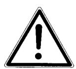
Be particularly aware of warning signs with this symbol, it marks measures that must be carried out in order to avoid accidents. The symbol appears in the instruction manual and on warning signs on the machine.
